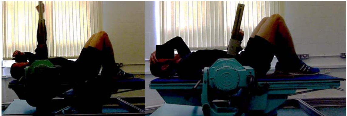
Figure 6.1. IsovLOCITY dynamometer configuration for ankle dorsiflexion (top left); hip flexion and extension (top right); shoulder flexion and extension (bottom left); and elbow flexion and extension (bottom right).
