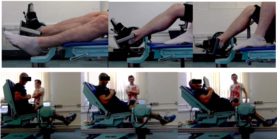
Figure 6.2. IsovLOCITY dynamometer configuration at three secondary joint angles each for ankle plantarflexion (top); and knee flexion and extension (bottom).
