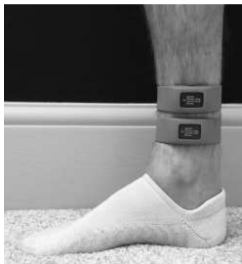
Figure 1 - positioning of IMeasureU Blue Trident sensors on the right shank.
